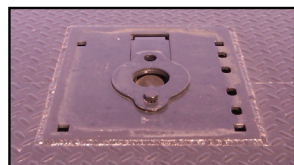
Retractable ball hitch for quick hook ups.
